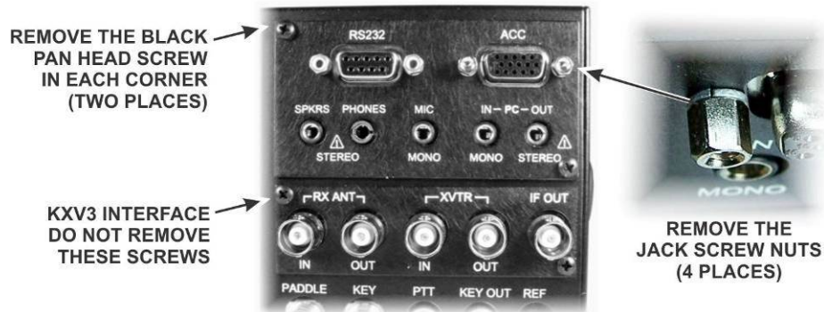
Figure 3. Removing the KIO3 Rear Panel Cover.
